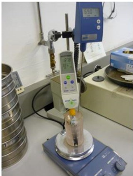
Photo 1: setup with sample immersed in caustic soda solution
