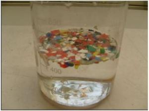
Photo 2: Sink float separation of regrind caps sample
