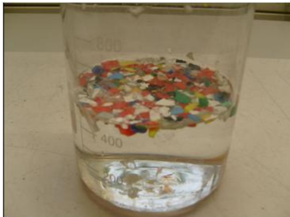
Photo 2: Sink float separation of regrind caps sample
