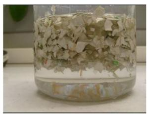
Photo 3: Sink float separation of regrind labels sample
