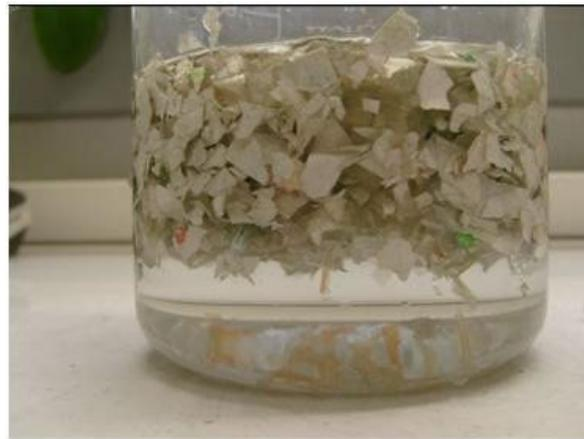
**Photo 3:** Sink float separation of regrind labels sample
