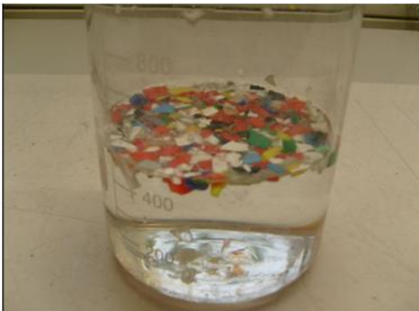
Photo 2: Sink float separation of regrind caps sample
