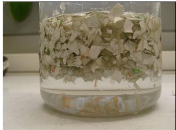
Photo 3: Sink float separation of regrind labels sample
