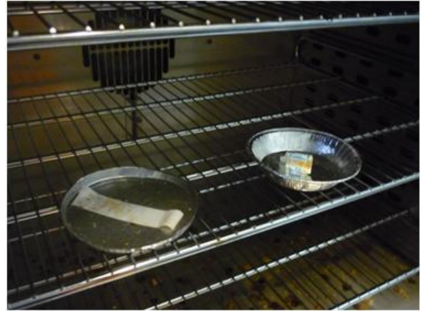
Photo 4: Dry sample for 2 hours at 80°C (W1)
