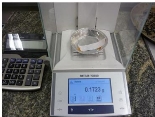
Photo 2: Analytical balance to weigh sample before washing (W1)
