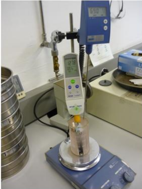
Photo 3: Glue removal setup with sample immersed in caustic soda solution
